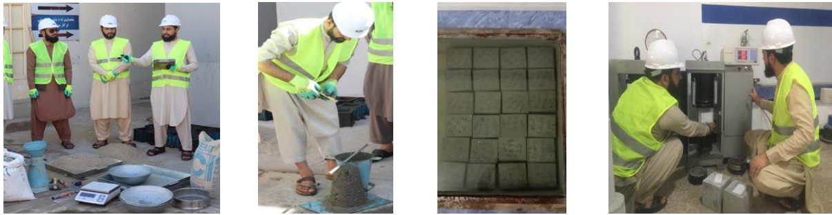
Figure 1. Shows mixing, slumping curing and compressive strength test.
